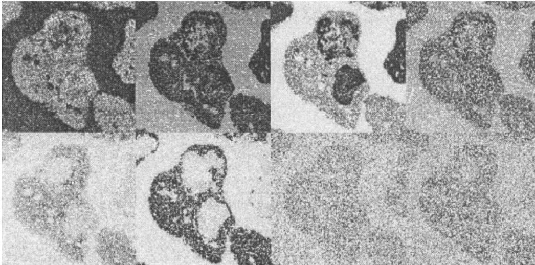
Fig. 2. Multi-spectral image with eight bands acquired by SEM/EDX method.
