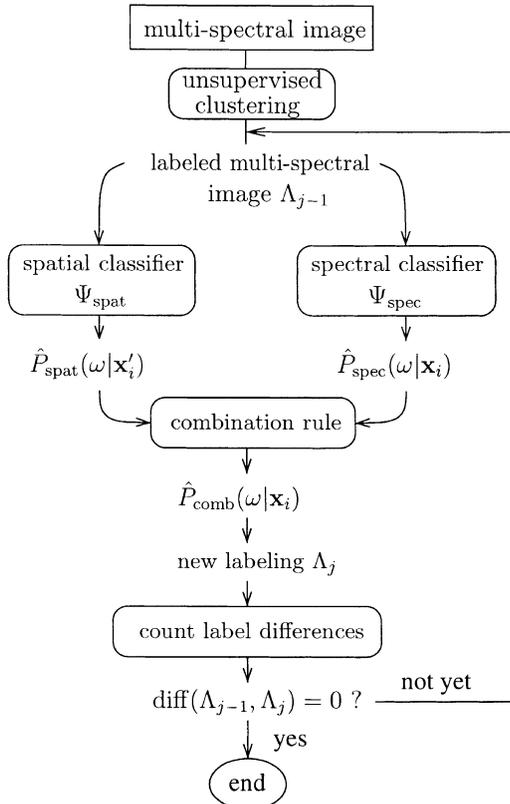
Fig. 1. The segmentation algorithm.
