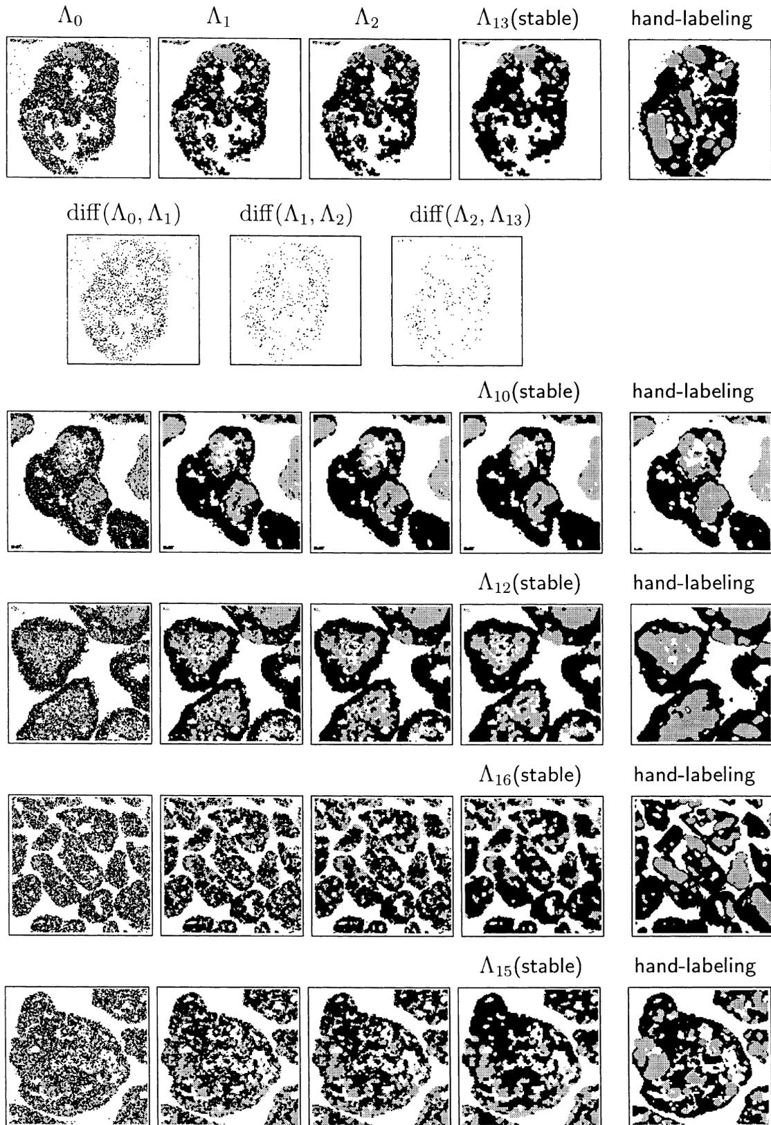
Fig. 4. Segmentation results for five multi-spectral images. For each image, initial labeling  $\Lambda_0$  is given together with results of first two iterations (label images  $\Lambda_1$ ,  $\Lambda_2$ ). Stable segmentations and hand-labeled images are then presented. For the first image, the differences between label images are also shown ( $\text{diff}(\Lambda_0, \Lambda_1)$ ,  $\text{diff}(\Lambda_1, \Lambda_2)$ , and  $\text{diff}(\Lambda_2, \Lambda_{13})$ ).
